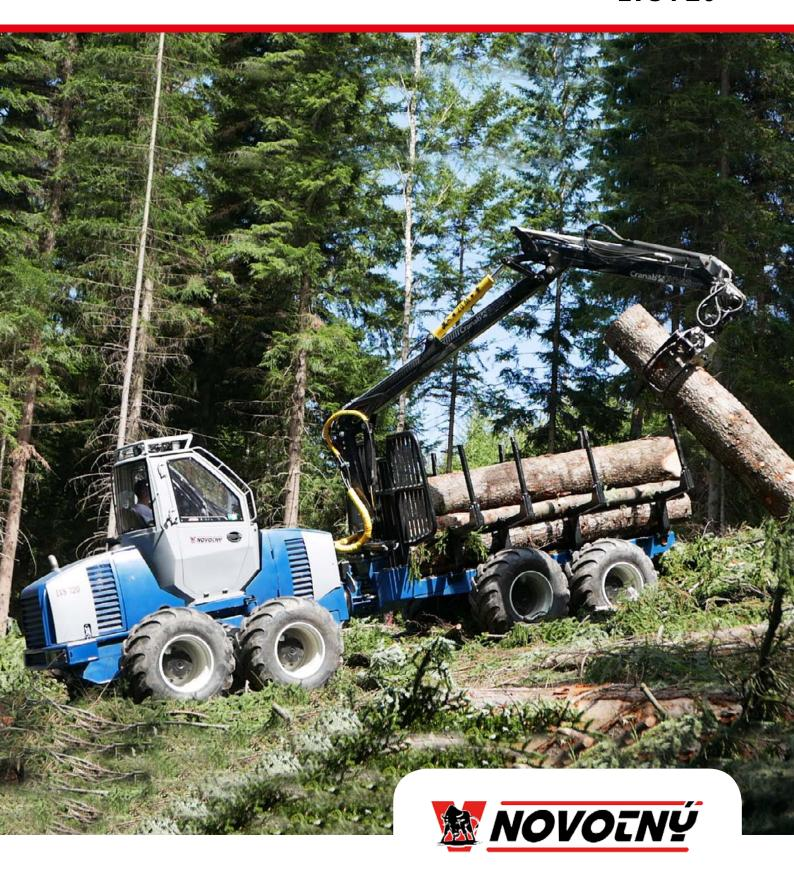
Powerful diesel engine • Robust NAF axles • High passing-through ability in dicult terrain • Traction 8x8 • Comfortable, 180° revolving cabin • Powerful and precise crane • Advanced electronic control system • Loading capacity 7500 kg • Machine width 2,2 meters
